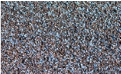
Poured In Place Rubber - PIP
